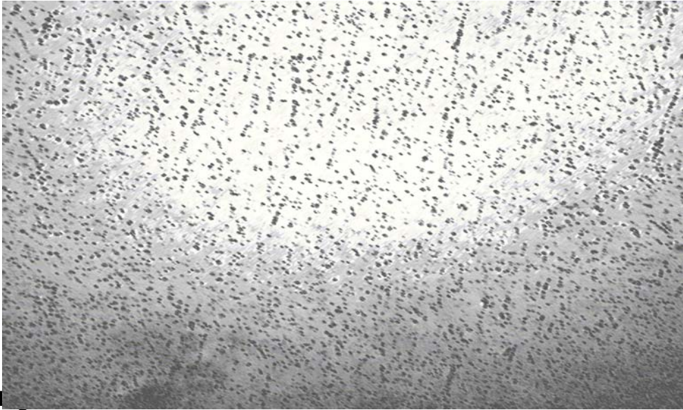
Figure 7. Zirconium weld structure after heat treatment, 750X
