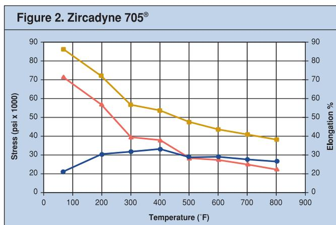
The ductility in both Zircadyne® alloys increases significantly with temperature. This improved ductility combined with a lower yield strength at 400°F provides improved conditions for severe forming operations.
